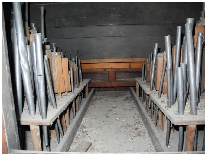
View through centre of 'M' layout of great soundboard
